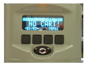
The screen displays "CARTRIDGE EXPECTED" if the RemoteLinc™ is installed when "ORIGINAL" cartridge type is selected.
