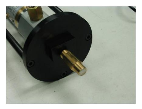
The other end of the RemoteLinc™ uses an o-ring for sealing.
