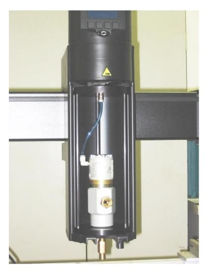
Note the blue pneumatic hose which transfers the ink feed pressure directly into the valve to control the on/off feeding just as it does with an ink cartridge. This air pressure opens the valve and allows the ink to flow. The valve closes via spring pressure when the air pressure is removed.
